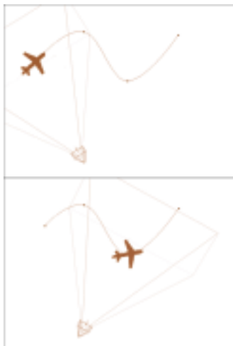
For example, if you link the camera to an airplane, the view of the scene will follow the airplane's trajectory as it moves along its motion path.
