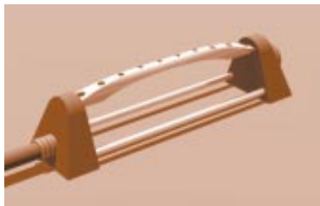
This sprinkler was created using compound Boolean operations.
